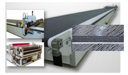
Pre-compaction steps are typical, which locally bond the individual layers together prior to preforming.
