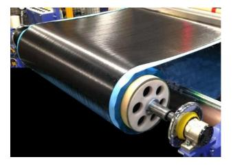
According to the designed lay-up sequence, unidirectional and/or woven prepregs are stacked as cut plies in predetermined angular directions or built up by a lay-up system. Such prepregs are either laid as single layers or processed as pre-laid multi-angle unidirectional layups. Often a thin glass fiber prepreg layer is placed in areas where the stringer is in contact with metallic parts to avoid corrosion.
