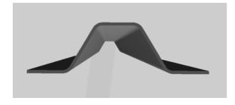
The typical shape of a fuselage skin stringer has a trapezoidal profile with 2 bases, similar to the Greek omega, which is where the name comes from. This shape allows the use of relatively thin stringers, which give the so reinforced skin the highest stiffening properties. Firmly attached to the skin, it forms a wide, stiff structure. Cold and hot
