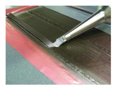
Ultrasonic cutting was originally developed for cutting prepreg materials by Design Technologies Limited, which became GFM in the mid-1980s. Today, ultrasonic cutting is used around the globe and is widely used for cutting prepregs, prepreg layups, dry technical textiles, honeycomb materials and many other materials.
