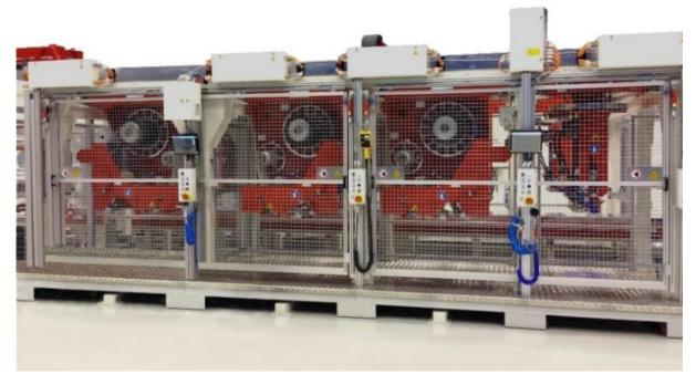
Alternatively, a combined system may be the right solution. In such a system, the unidirectional prepreg is laid lengthwise by a laying head and the angular strips are cut just in time by a cutting machine and placed at the programmed position by a pick & place system.
