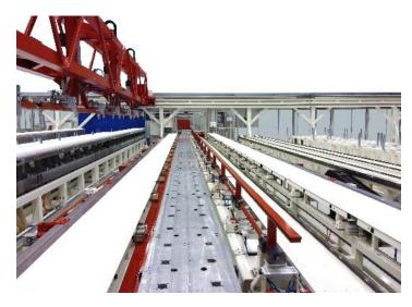
Optimized handling solutions are important for proper serving the various stations in an automated stringer manufacturing cell. Handling starts when raw materials enter the cell and is required for the transfer of semi-finished products from one manufacturing station to the next or finished stringers to storage or output stations. An optimized handling system also provides the right tools at the right time at the different stations, serves buffer or tool stations and
